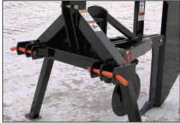
CAT. I AND II HOOKUP PINS Cat. I and II hookup pins for easy 3 point hookup or quick attach skid loader mounting plate for easy mounting.
