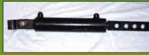
HTL-1055 HYDRAULIC TOP LINK CYLINDER The hydraulic top link cylinder (required for 3 pt hitch mountings) goes in place of the rigid top link on the tractors 3 pt hitch. This allows the operator to adjust the pitch of the knife on the machine so it doesn't nose dive or try to come out of the ground.
